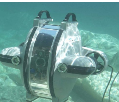
Scout ROV with patented pitching system
